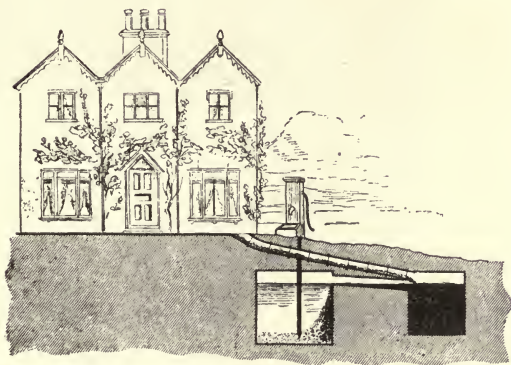
Fig. 593. New Vicarage Cesspool overflowing into a Tank.
